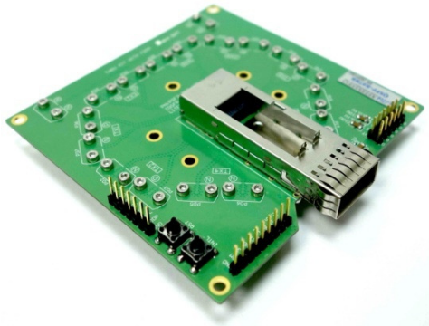
Fig 1: QSFP Receptacle Test Fixture(QSFP-B07BR)
